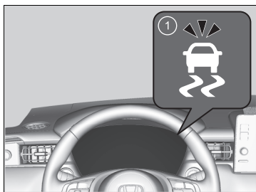
① VSA System Indicator
